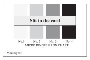
Opacity is measured from an observation point between 30 and 400 metres from the emission point. The observation point must allow full view of the emissions. The sun must be oriented in the 140° sector to the observer's back. The observer must make observations using a line of vision that is perpendicular to the direction of the plume.
