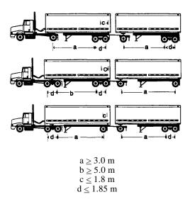
A.87Any combination of road vehicles forming a Type C double train with 8 axles, 6 of which form 3 tandem axles, composed of a tractor, a semi-trailer and a trailer with a double drawbar dolly and meeting the specifications of class A.86, as shown below, belongs to this class:
