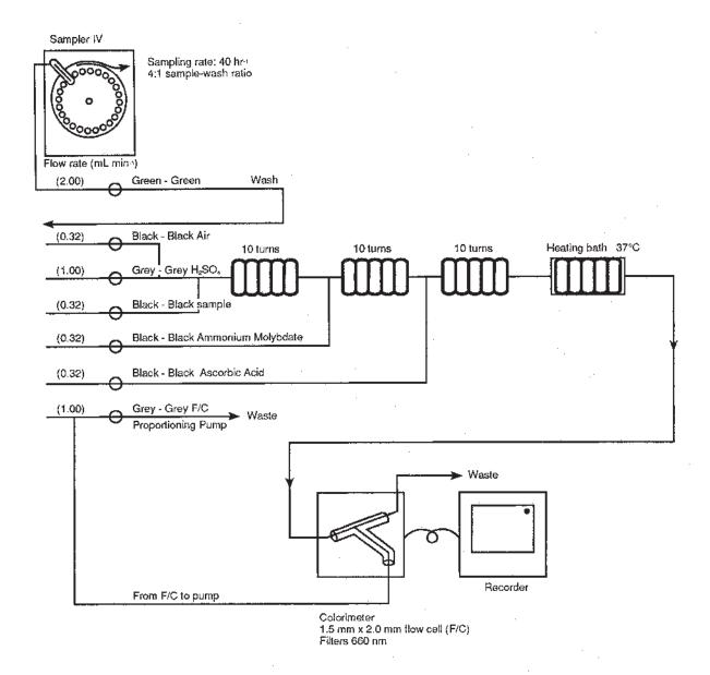
Figure 1. Flow diagram for the automated analysis (Technicon AutoAnalyzer) of P in Me lich III soil extract
