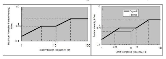
The employer must use, according to the manufacturer's instructions, a seismograph to monitor the velocity of particles to ensure the compliance of the results with table 2.6.1 or graphs 2.6.2 as provided above. The method for monitoring vibrations and the calculation of frequency must be approved by an engineer.
