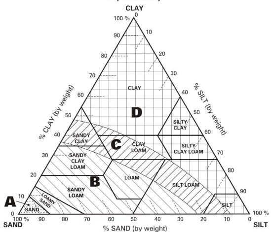
SAND : A soil separate consisting of particles A: High permeability zone between 0.05 mm and 2 mm in diameter
