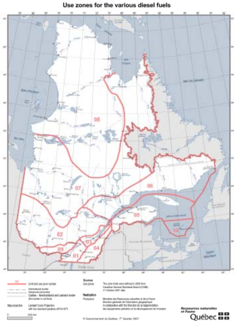
FIGURE I MAP ILLUSTRATING THE LIMITS OF USE ZONES OF DIESEL FUELS ACCORDING TO THE AVERAGE 2.5% LOW-END DESIGN TEMPERATURES
